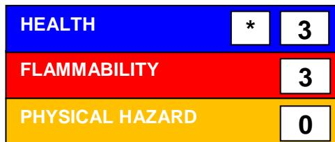
HMIS® ratings are based on a 0-4 rating scale, with 0 representing minimal hazards or risks, and 4 representing significant hazards or risks. The "\*" represents a chronic hazard, while the "/" represents the absence of a chronic hazard.
