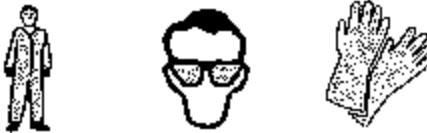
Wear overalls, safety glasses and impervious gloves. Avoid breathing dust when sanding. Wet sand or use a dust mask. Always wash hands before smoking, eating, drinking or using the toilet. Wash contaminated clothing and other protective equipment before storage or re-use.
